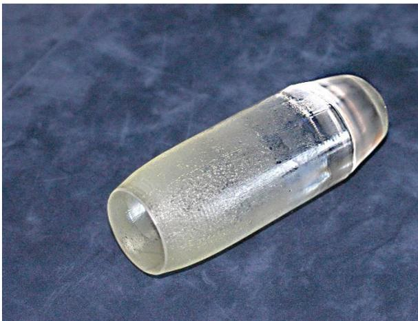
*Figure 9 Photo of the Zr-codoped YAP:Ce single crystal (45 mm in diameter and 125 mm in length). Courtesy of the CRYTUR company.*
